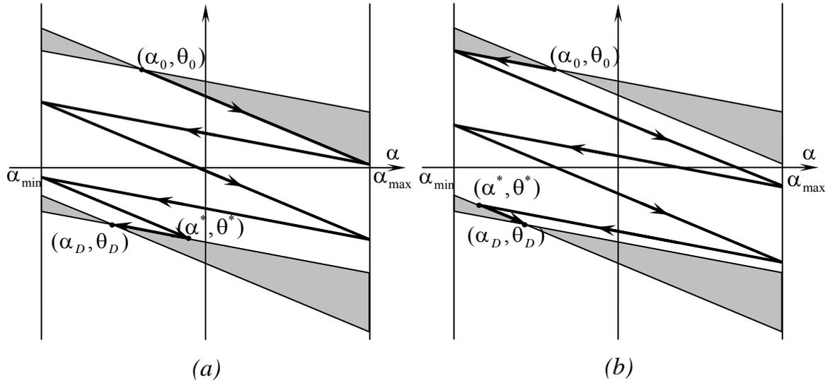
Figure 3. The trajectory of the imaging point for the case when its final position lies below the attainability domain from the initial position
