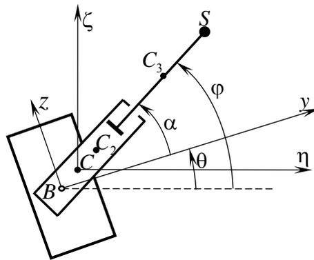
Figure 1. The constructive scheme of the space robot
