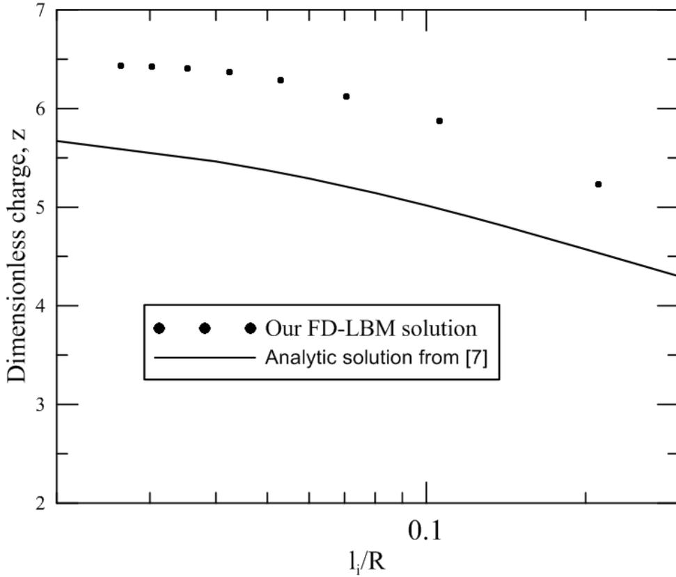
Figure 2: Dimensionless grain charge  $z$  as a function of the ion mean free path  $l_i$  normalized to the grain radius  $R$  for  $\lambda_D = 2R$ . Line—analytic solution from [7], dots—our numerical FD-LBM.
