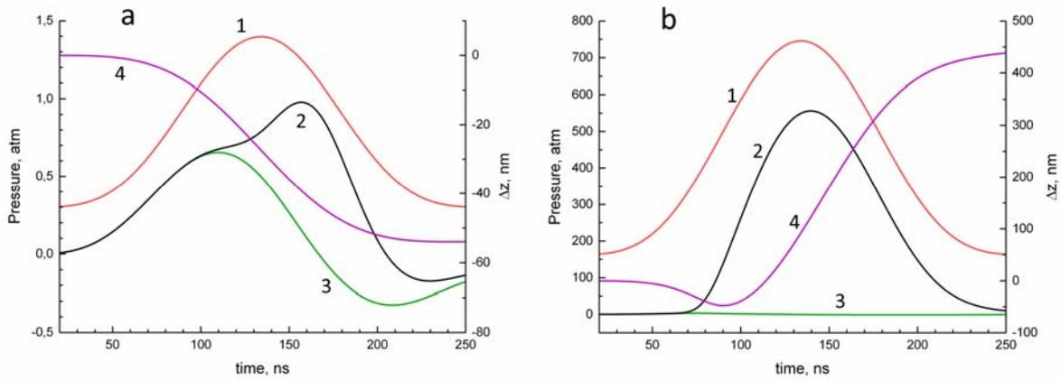
Figure 1: Time dependence of thermoacoustic pressure part (3), total (including vaporization) pressure (2) and irradiated surface displacement  $\Delta z$  (4) during laser pulse (1) action at different fluences  $E = 20$  (a) and  $200$  (b)  $\text{mJ}/\text{cm}^2$ .
