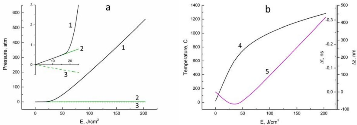
Figure 2: Maximum values of the total pressure (1), its thermoacoustic component (positive 2 and negative 3), surface temperature (4), and surface displacement value  $\Delta z$  at  $t = 200$  ns (5) versus laser fluences.
