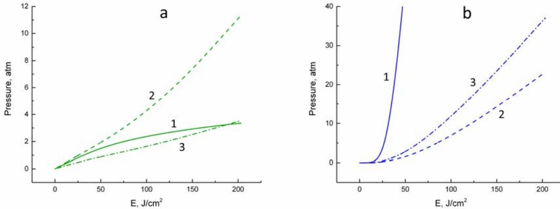
Figure 6: Maximum values of the pressure component: smooth (1) and modulated (2, 3), thermoacoustic (a) and vaporisation (b) versus laser fluence  $E$ .
